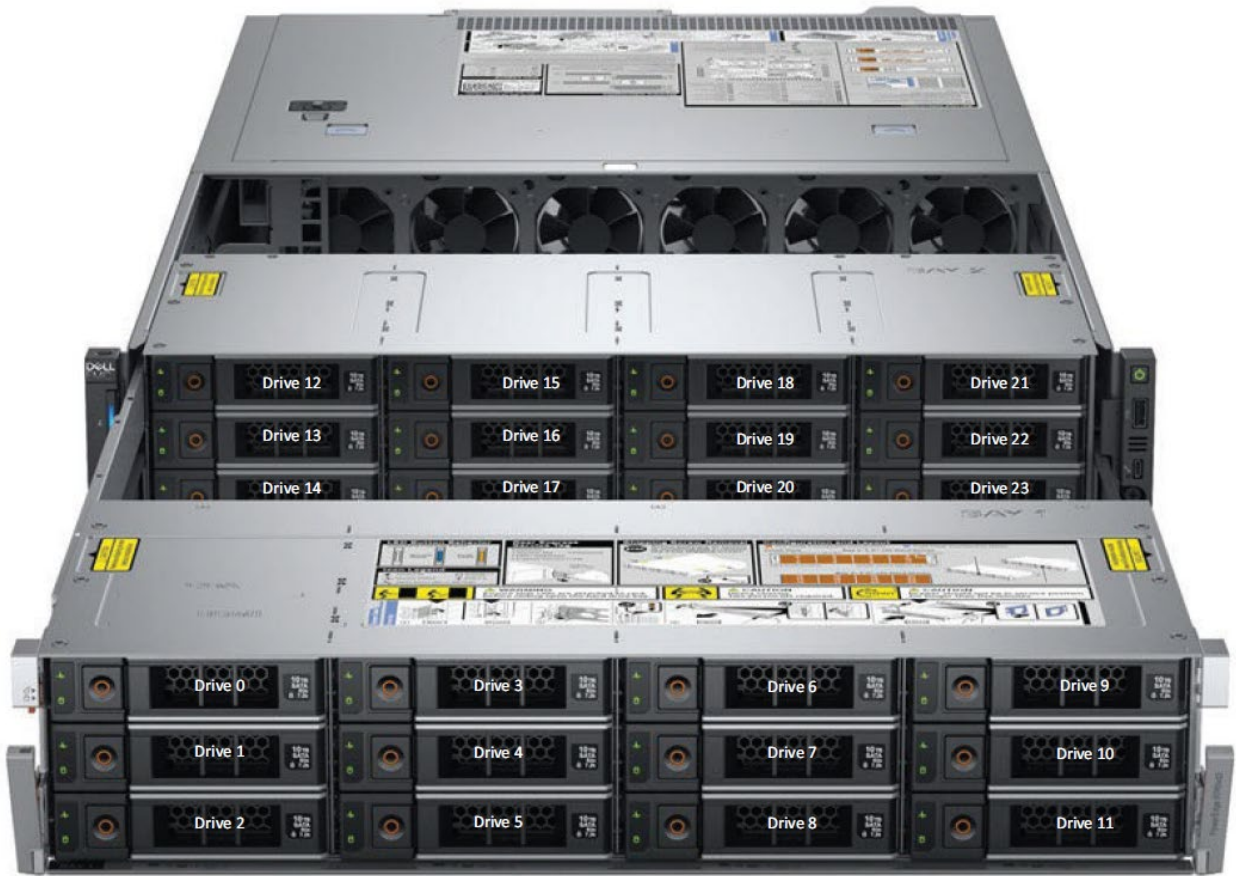
Figure 4. View of drive bay extended
