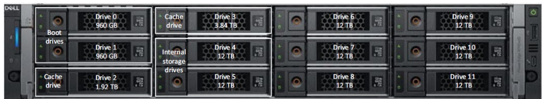
Figure 2. Front disk layout (drive bay 1)
