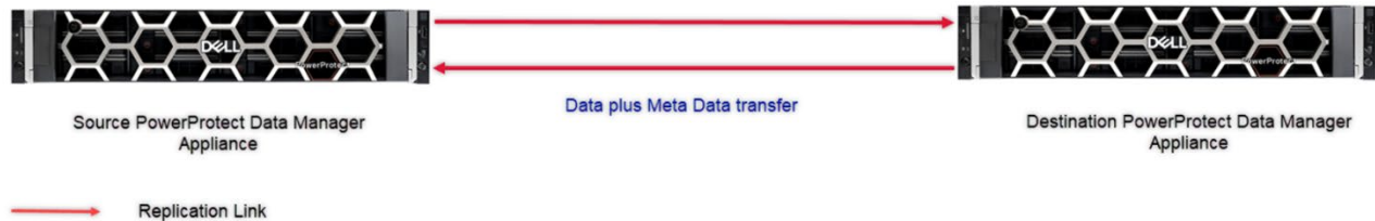
Figure 18. Bi-directional replication topology of PowerProtect Data Manager Appliance
